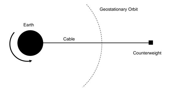
The section of cable below the geostationary orbit would fall to Earth under the influence of gravity. Beyond the geostationary orbital radius the gravity field is weaker and the cable, with added counterweight, keeps the cable held up, under tension.
