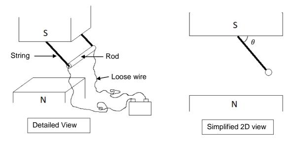
When everything is connected, the rod swings to one side and remains in the position shown in the simplified 2D view.
