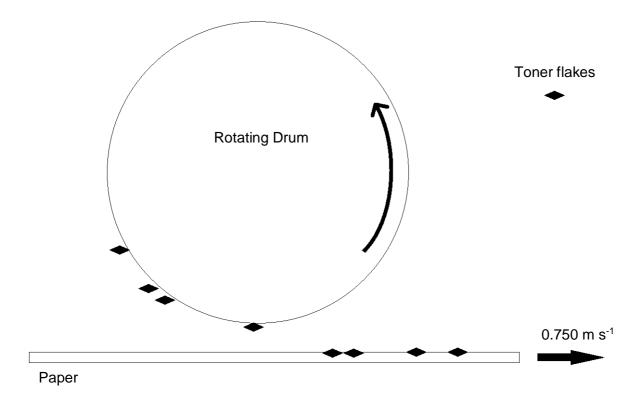
The diagram is not to scale and exaggerates elements of the design to make it clear. The drum is 4.50 cm in diameter. The minimum distance between the drum and paper is 50.0  $\mu$ m. Each flake of toner is 1.89 × 10<sup>-8</sup> g. The paper moves past the drum at 0.750 m s<sup>-1</sup> and the drum rotates at the same rate so that it can print clear images onto the paper as they move past each other.
